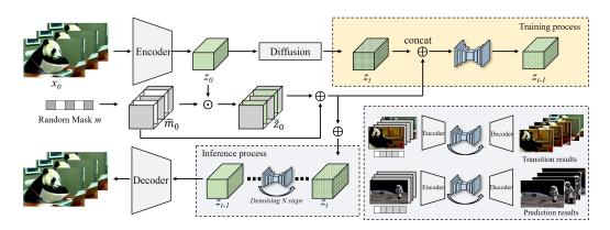
Figure 4: **Overview of our proposed method.** We present our S2L generation model for generating transition video and long video prediction. Our model supports text as input, which is processed through a clip encoder and injected into the model (blue part). For brevity, we omit the details of the text injection, which is identical to the stable diffusion model.
